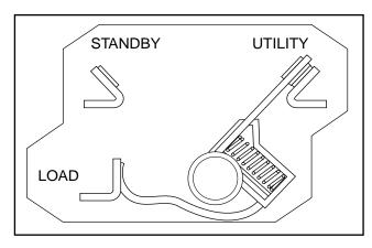
Figure 2. Load Connected to Utility Power Source
